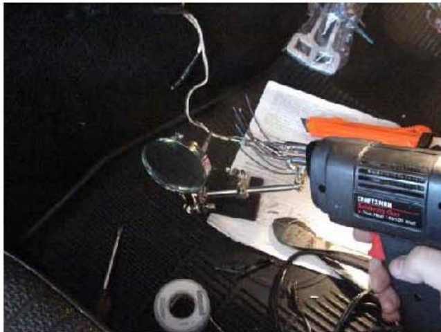
The cool Harbor Freight clamp helped hold the speaker wires in place during soldering.
