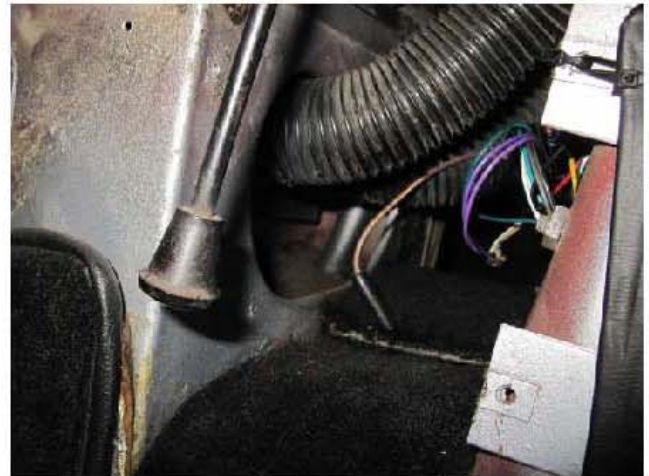
Due to its shorter depth, the new stereo no longer fouls the vent tubes. Defrosting should be better!
