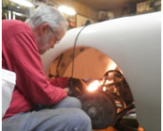
Hammer against Hammer breaks the steering arm free
